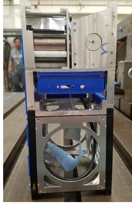
Figure 3. Prototype of DMD with CubeSat Structure
